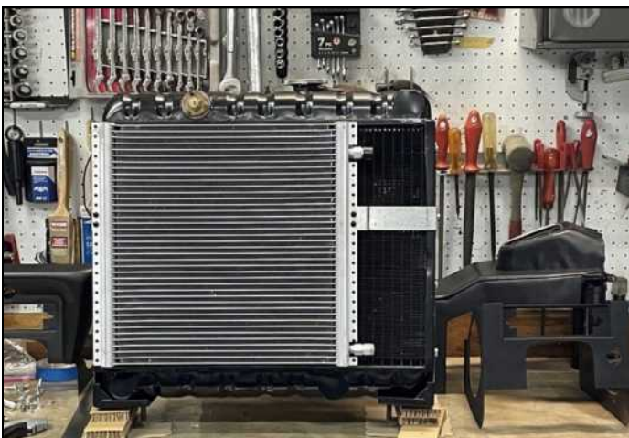
Left: Condenser on E-type radiator
