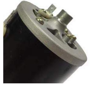
Mort Resnicoff, New Jersey: I have installed an alternator to replace the generator and regulator. It is from a company in England called Accuspark. They call it a Dynamator and it is built in the body of the standard TD generator. The car is running fine but my ammeter is erratic.
